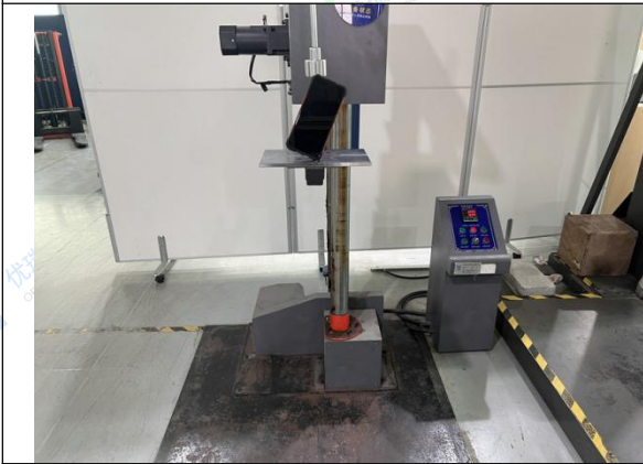
Fig.54: Test setup corner
