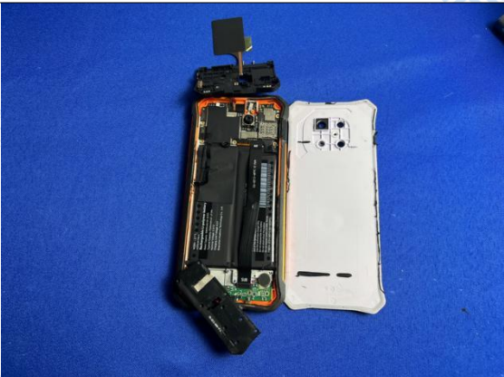
Fig.18: Disassembly Inspection after test
