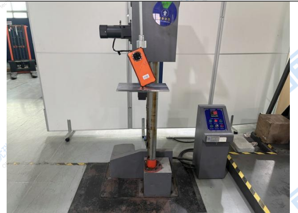
Fig.59: Test setup corner
