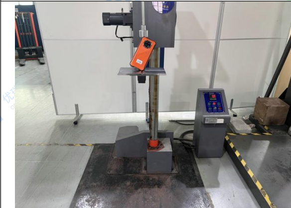
Fig.58: Test setup corner
